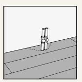
Mark the centre point of the pipes on the plank. Drill holes 20 mm bigger than the pipe's diameter (if gap distance selected is 10 mm). Cut according to the picture. Fix with white glue and replace the floor pieces. Cover the holes with pipe collars or fill with a joint sealer.
