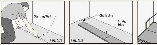
Using the starting wall as reference, snap a chalk line on the subfloor at distance X from the wall as shown in Fig. 1.1. Align the straight edge with the chalk line and secure it to the subfloor.
