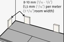
We recommend a clearance to the wall of min. 8-10 mm (1.5 mm per meter room width).
