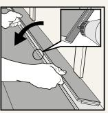
Remove the locking element/hook according to the picture. Use white PVAc glue to connect the planks. Position wedges between the glued plank and the wall.
