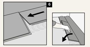
Second plank, second row. Place the plank gently and tightly to the short end of the previous plank. Lower the plank down in a single movement. Make sure the planks are tight against each other. Press down the plank.
