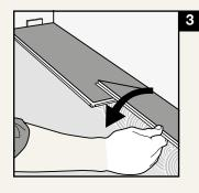
Lower the plank down in a single movement. Make sure the planks are tight against each other. Press down the plank.
