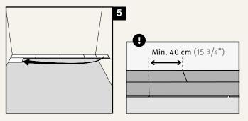
Start the second row with the offcut from the first row. • Note! There must be at least 40 cm between the short end joints of the planks.
