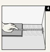
At the end of the first row, put a wedge to the wall and measure the length of the last plank to fit.
