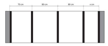
Always put a support in the corners. The distance from the left corner to the center of the next support is 70 cm. From then on, put supports every 80 cm (center to center)
